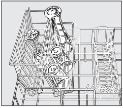
The insert for glasses can be fitted in the left or right of the bottom basket in place of a removable insert. Very tall glasses can be held more securely by the vertical supports.
